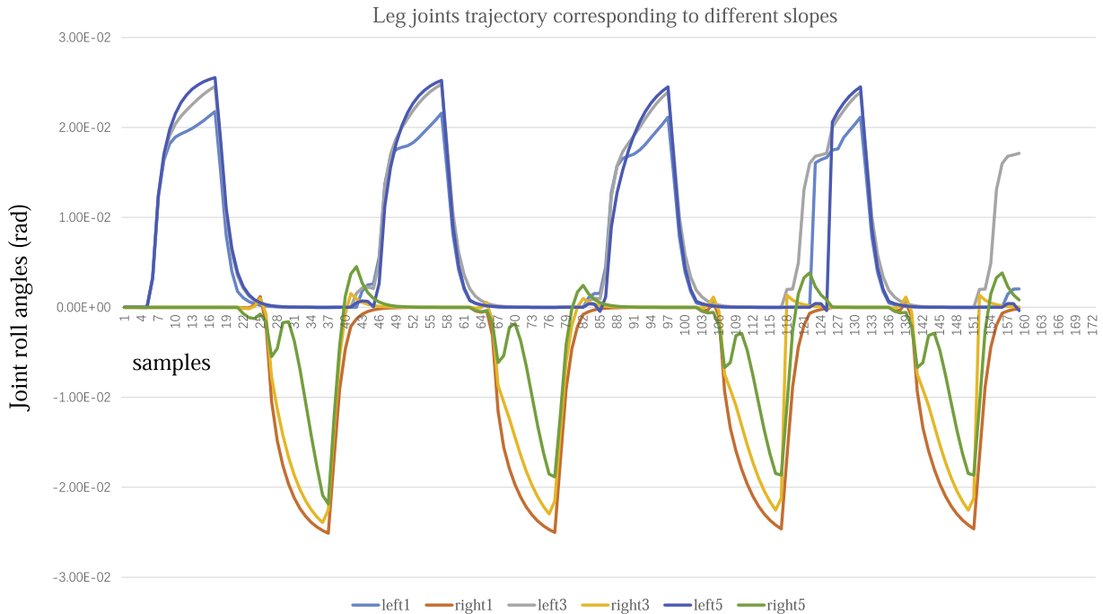
Fig. 12. The roll angle trajectory of both legs under different slope in 1, 3, 5 degree.
