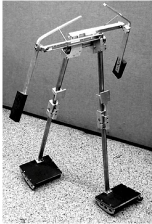
Figure 3.5: A passive dynamic walker by Collins [28].
