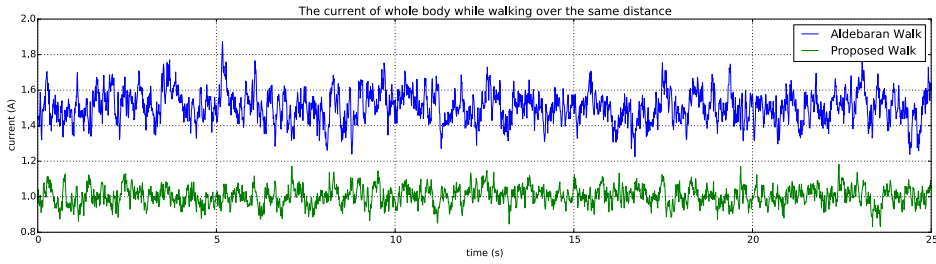
Figure 5.16: The whole body current of a Nao after walking 0.75 meter with the step length 3.6 cm. The lines represent the unfiltered current values from two different walking gait. Note that the mean value of our proposed walk is clearly lower than that of the Aldebaran walking gait
