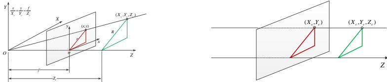
Fig. 1: Perspective camera model Fig. 2: Orthographic camera model
